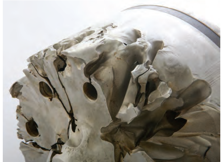
Fully stellited cage guided trim after two weeks operation
