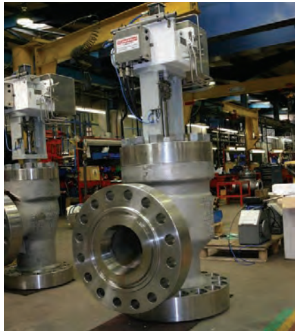
12" ANSI 1500 choke C/W electro-hydraulic actuator
